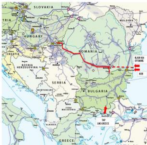
Figure 8– The interconnection points of the Romanian gas transmission system with the similar Bulgarian and Hungarian systems
